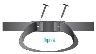
2. After the strap is completely laced through the mounting base, make a loop with the strap, where it runs across the middle of the base as illustrated in figure 6. This loop is necessary to access the two mounting holes in the base.
